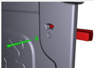
Hold the Armal key in place to lock the outer screw
