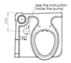
Insert the hand pump from inside the tank
