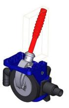
Mount the pipe in the pump outlet (lenght xx cm)
