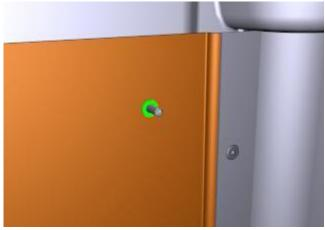
Pull out the rivets from the outside of the restroom
