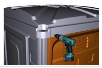
Insert the rivets from the outside of the restroom
