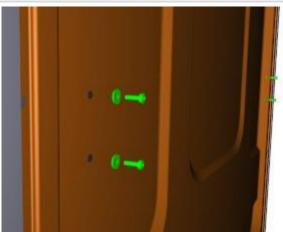
Secure the handle on the inside of the restroom with No. 4 self-blocking nuts and washers
