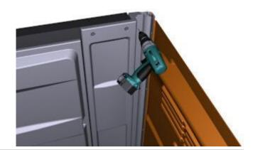
Insert the rivets from the inside of the restroom
