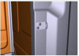
Install two plates on the horizontal handle poles
