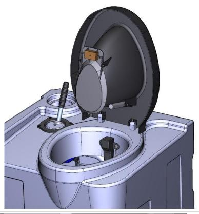
Assemble the bowl with the metal bar and the radial stop ring
