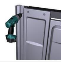
Insert the rivets from the inside of the restroom
