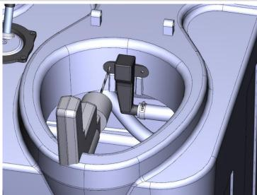
Fix the nozzle with No. 2 rivets
